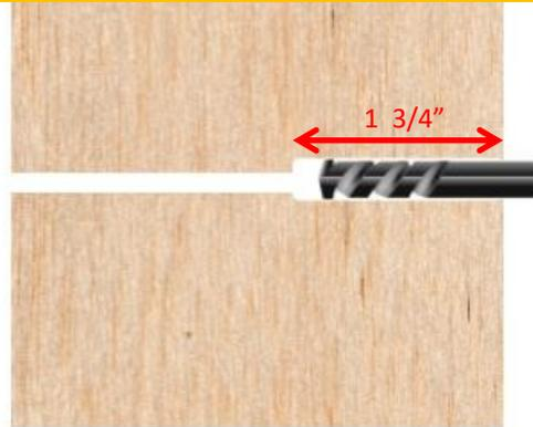
**3** Start on the "Tensioner End". Push the swaged threaded bolt through 1/4" hole in post. Slip on washer and thread nut on to threaded bolt. This is how cable will be tensioned later.
