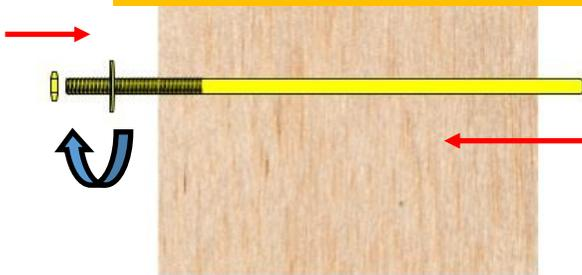
**4** String cable through all line posts down to other end. Slip washer on to the "Pull-thru Lock" fitting and push cable through, twisting the cable clockwise as you get it started. Once cable is through fitting, pull cable tight by hand while pushing the fitting into the countersunk hole in end post.
